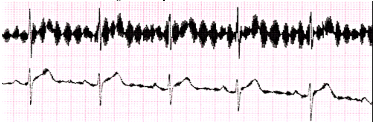
Figure 19 Sixty Hz electrical interference
